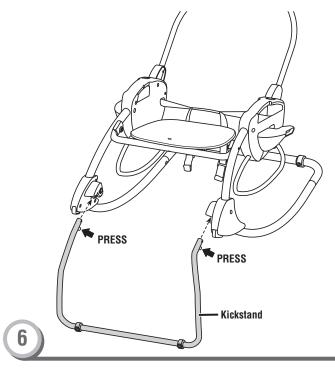
• While pressing the tab on each end of the kickstand, insert the kickstand into the small tube inside each side rail.
